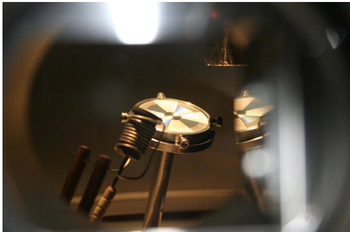
Image of a multicomponent target in the PLD vacuum chamber.
