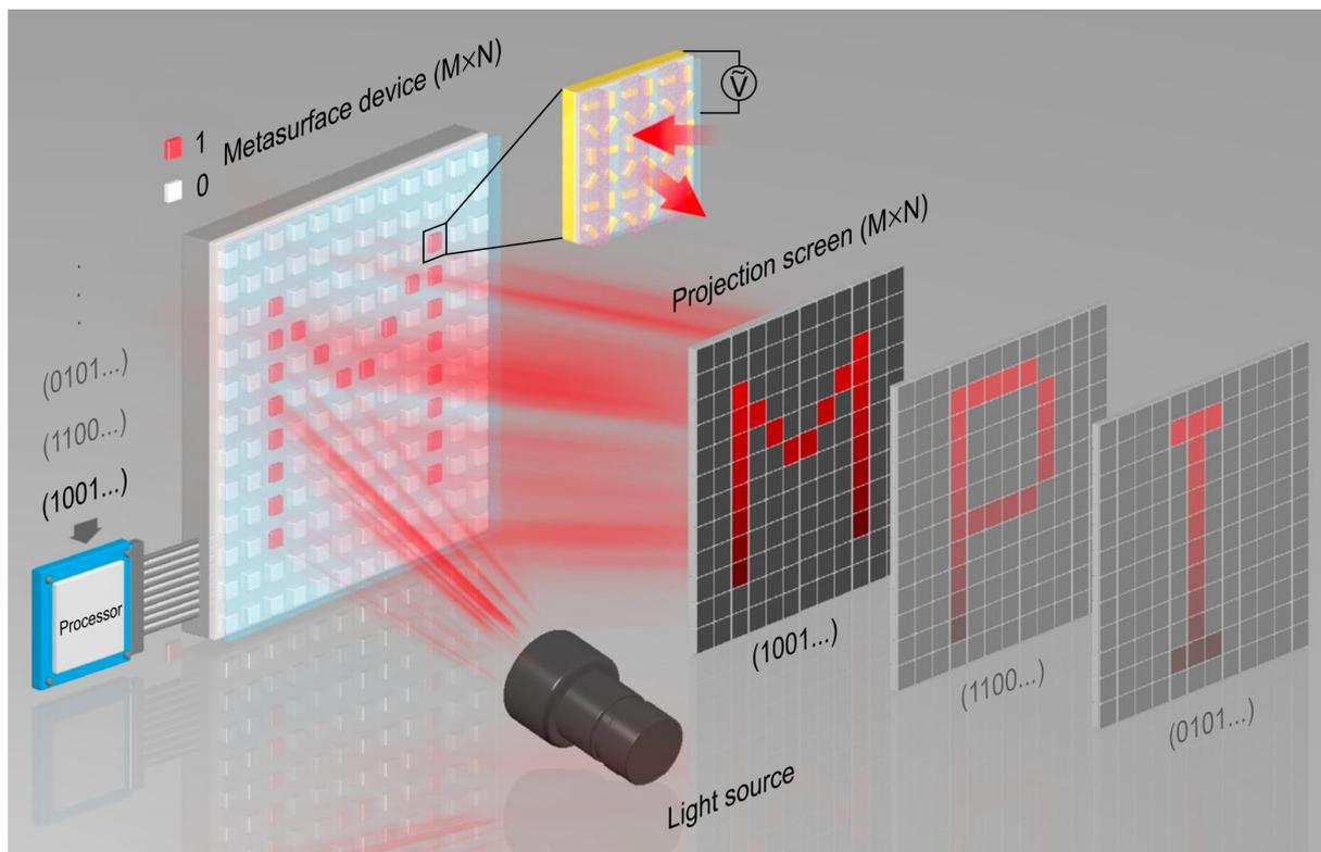
**Fig. 1:** Possible implementation of the invention. A digital metasurface device for light projection displays comprises metasurface pixels in an  $M \times N$  array. The intensity of the reflection from each metasurface pixel is controlled by an addressable electrode and can be independently switched on and off. Programmable images ( $M \times N$  resolution) are dynamically displayed in the far field.
