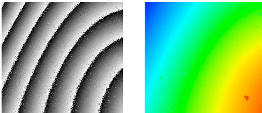
**Figure 2.** Result of a speckle deformation measurement, physical averaging applied. Left: Raw phase. Right: Unwrapped phase, obtained via the same standard, unsophisticated unwrapping algorithm.
