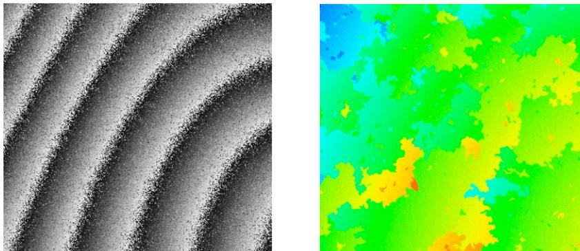
**Figure 1.** Result of a speckle deformation measurement. Left: Raw phase. The huge number of phase singularities makes the raw phase appear noisy. Right: Unwrapped phase, obtained via a standard, unsophisticated unwrapping algorithm. The errors during unwrapping completely mask the systematic phase from the deformation.
