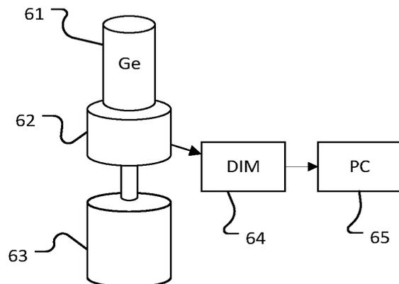
Fig. 2: The gamma detector comprises a large Germanium diode, an amplifier and a cooling
