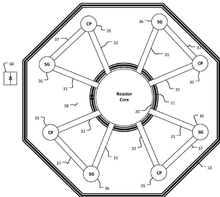
Fig. 3: The detector assembly can (60) can be operated outside of the biological shield (10). Gamma rays from the main cooling cycles including pumps and steam generators (31-37) are being detected even at larger distances.
