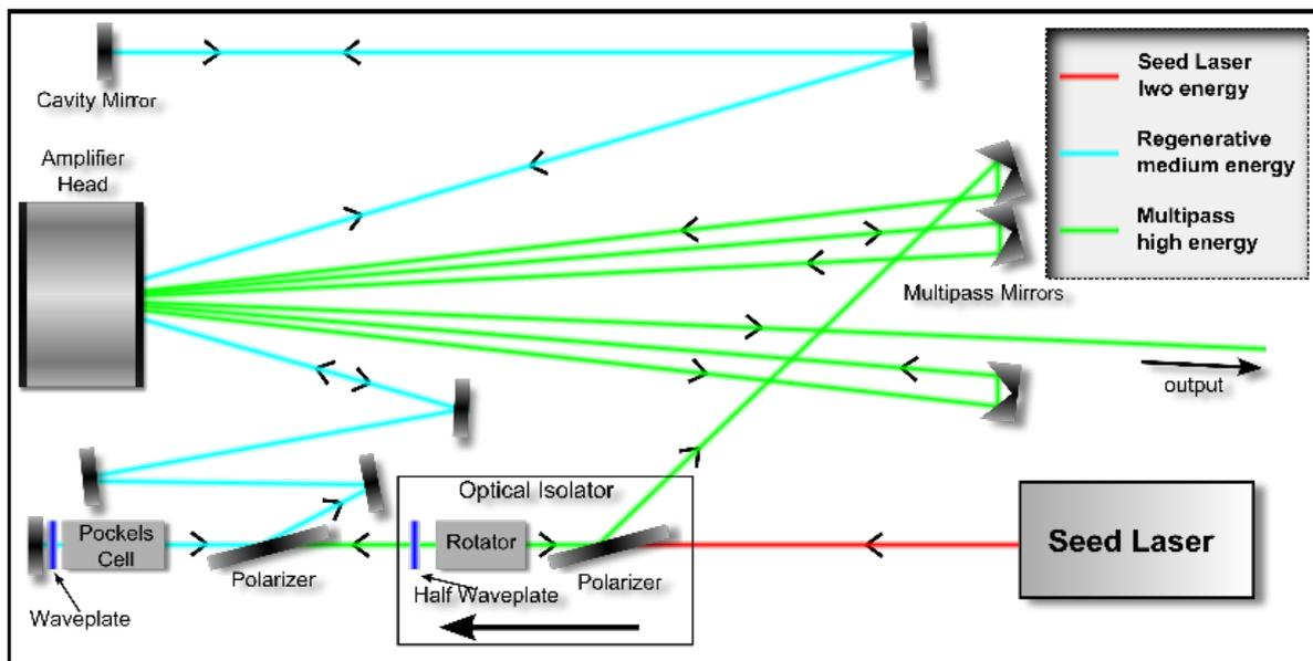
Figure 1: Schematic picture of the invention. The different sections are marked in red, blue and green. Red: Seed beam with low energy. Blue: Amplification in the regenerative amplifier. Green: High-energy multipass amplification.
