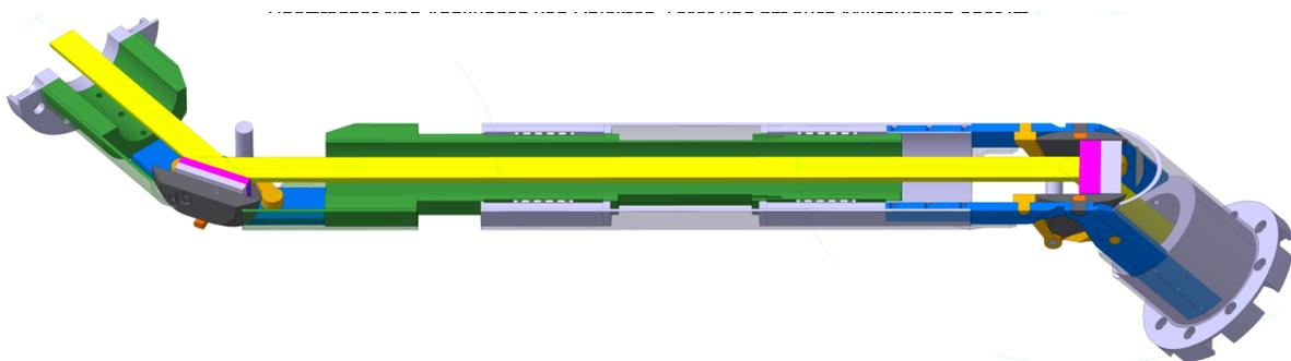
**Figure 1:** Schematic illustration of the movable beam guide with articulated mounting legs (colored blue), beam guiding parts (colored gray/green) and the movable coupling unit/joint (colored black). The yellow line shows the beam path, which is automatically tracked by precisely aligned mirrors (colored purple). The movable beam guide combines flexible joints with a rigid guide to provide low-loss deflection of the beam at different positions.
