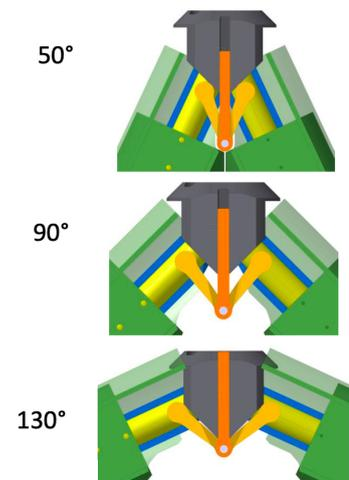
**Figure 2:** Reflector articulation shown with adjustable 2" mirror at different aperture angles (50°, 90°, 130°). Automatic beam tracking is achieved by mechanically coupling the coupling arms (colored orange) to the articulated mounting legs (colored blue) and the movable coupling unit/joint (colored black). The reflector/mirror is mounted on the movable coupling unit. At any aperture angle the incoming light is reflected into the outgoing arm of the beam guide.
