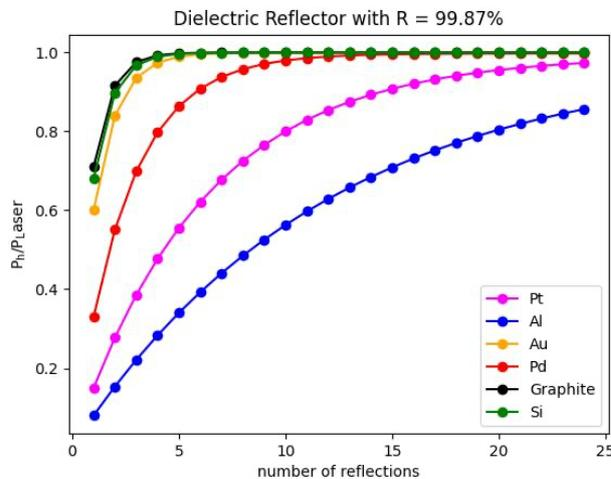
**Figure 2:** CELAH heating efficiency for different reflective (metals) and non-reflective (Si, Graphite) samples as function of reflections off the sample surface using a dielectric reflector with >99.8% reflectivity. In this configuration, almost all laser power can be provided as sample heating power.
