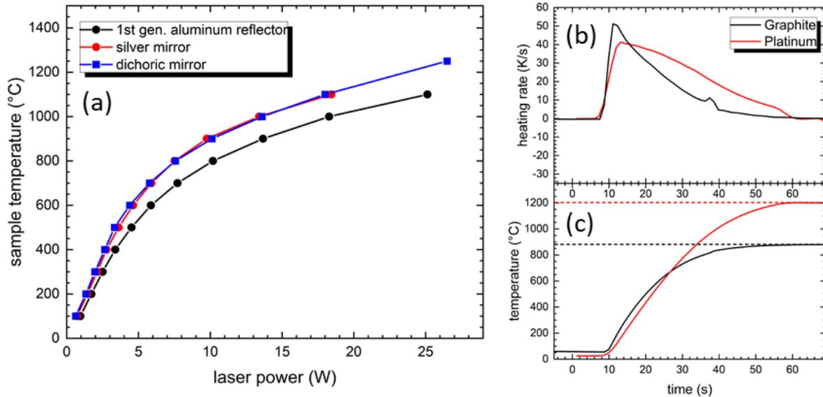
**Figure 4:** (a): Platinum sample temperature in dependence of the applied laser power for different CELAH system designs. (b) and (c): Heating rates for heating of platinum or graphite from room temperature to 1200°C and 900°C, respectively.
