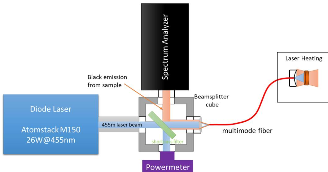
**Figure 5:** Scheme of the laser heating system with integrated optical temperature measurement and online tracking of the laser power.
