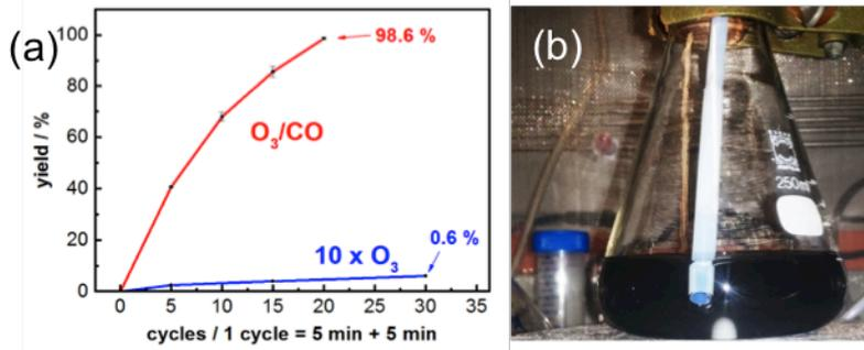
Fig. 2: (a) Pt Black powder suspension Pt yields of CO/ozone and pure ozone treatment in 0.3 M HCl + 1 M NaCl at room temperature. Images of before (b) and after (c) complete dissolution (yellow) of Pt suspension after 20 exchanges between ozone and CO.
