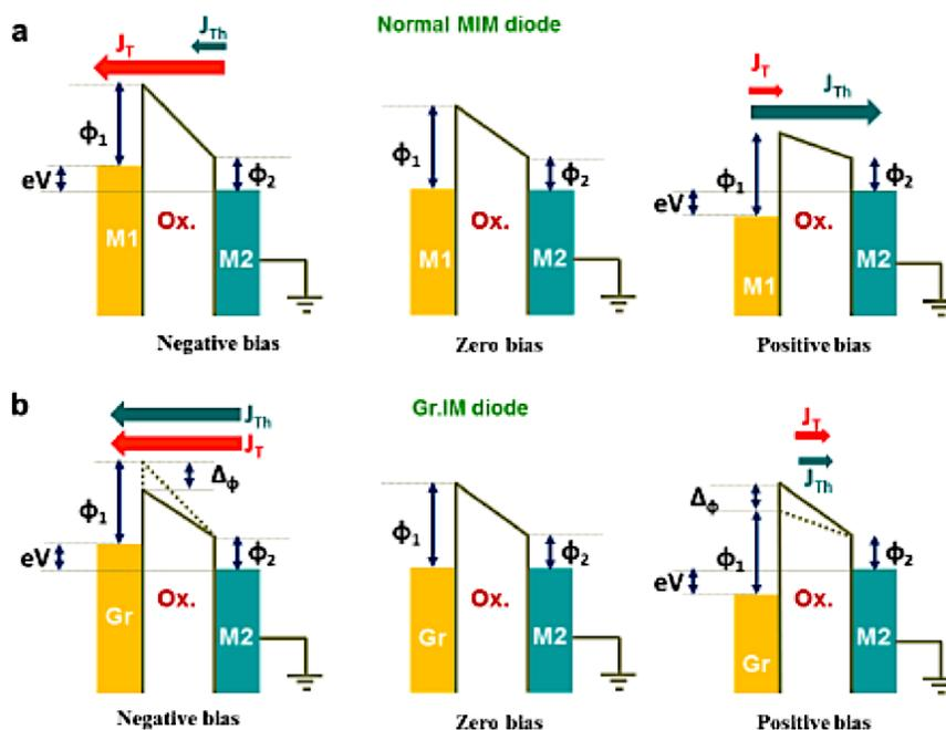
Fig. 1: Operation principle of (a) a conventional MIM and (b) a GrIM diode.  $\Phi_1$  and  $\Phi_2$  corresponding to the difference between the work function of metal electrodes and the electron affinity of the oxide insulator.  $J_{Th}$  (blue-green arrow) and  $J_T$  (red arrow) denote the thermionic emission and tunneling current, respectively.
